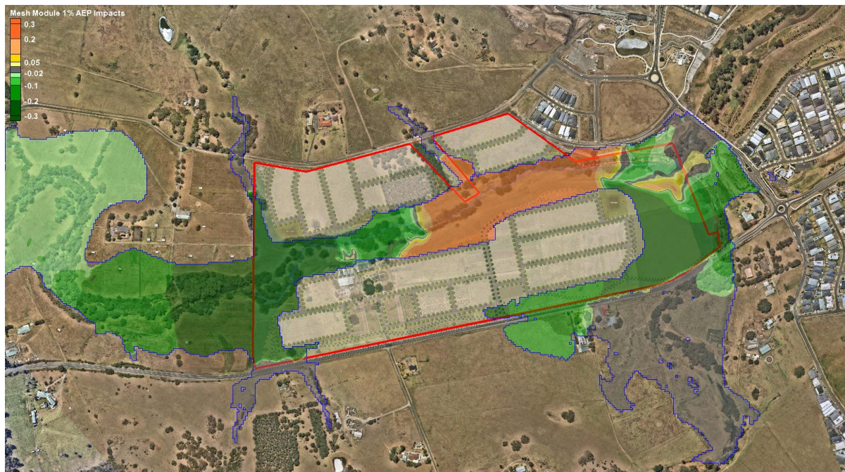
Figure 5.3-1 1% AEP Peak Flood Surface Level Impacts
